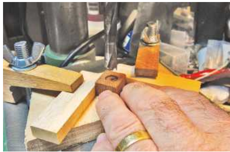
▲ Pic.11 A simple jig consisting of two strips clamped to the drill platen will enable you to get consistent beads
